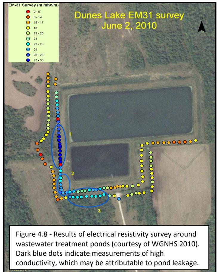
Figure 4.8 - Results of electrical resistivity survey around wastewater treatment ponds (courtesy of WGNHS 2010). Dark blue dots indicate measurements of high conductivity, which may be attributable to pond leakage.
